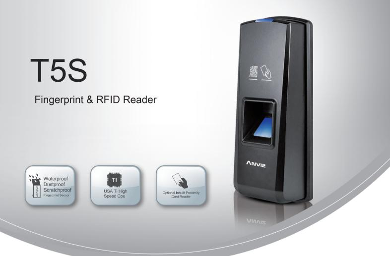
T5S is an innovative fingerprint card reader which fully integrates fingerprint and RFID technology. The very compact design makes it suitable for installation on door frame. T5S has standard RS485 output to connect with ANVIZ whole access control production to be a dispersed type access control system. T5S can easily update the existing card readers for higher security level of fingerprint and card.
